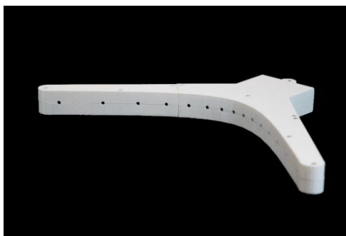
Figure 1. Prototype of the 15-channel 2-dimensional microphone array placed in front of the child, with approximate dimensions of 0.4 m x 0.13 m (WxL).
